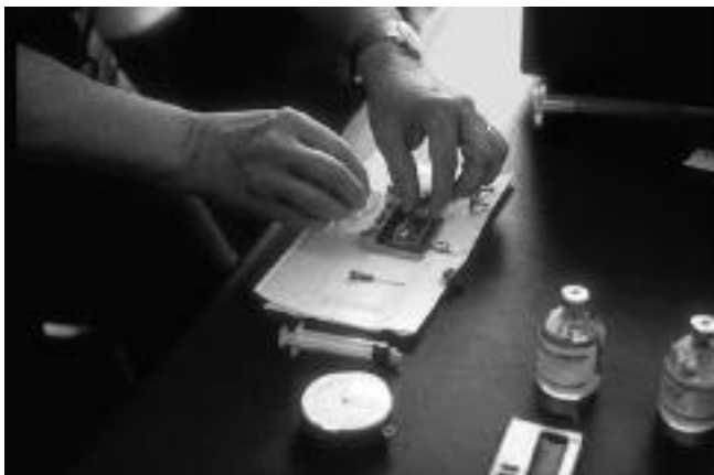
Sample cell, being dried between measurements. Note also needle and syringe ready for discard. Each was used but once.
